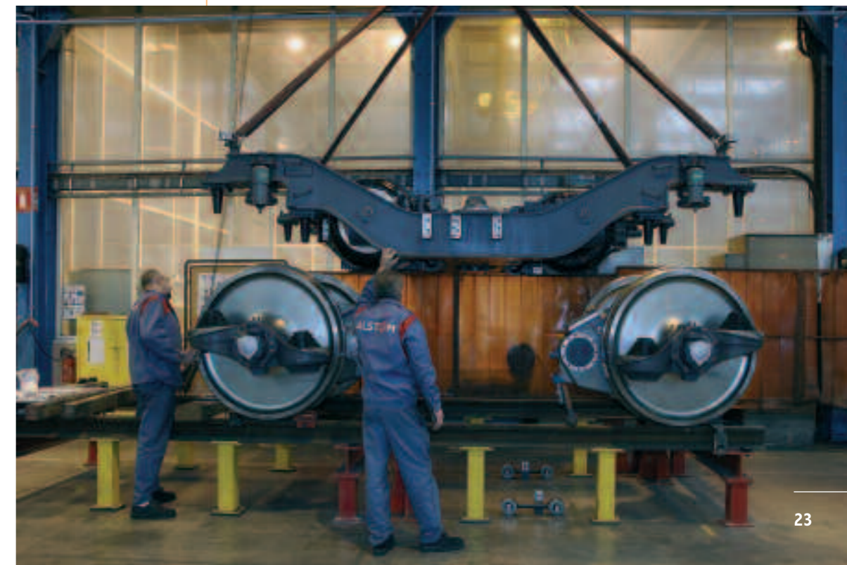
TGV motor bogie being mounted at Alstom plant
