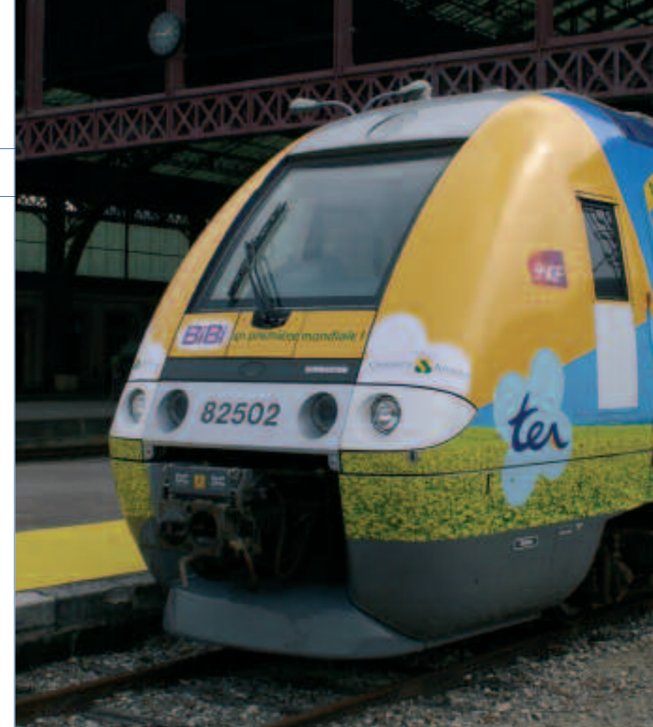
The BiBi AGC developed for operation in electric or diesel mode depending on the lines used, will revolutionise regional transport.
